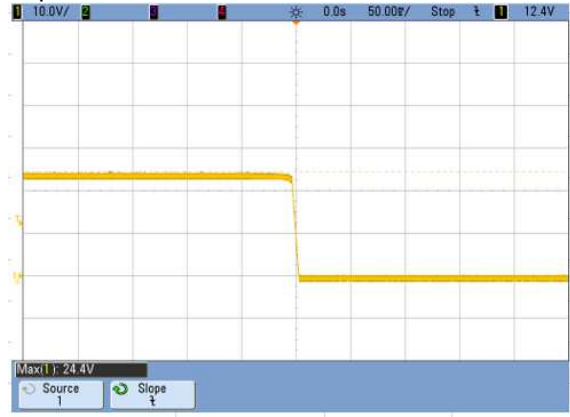
Output turn-off rated load
